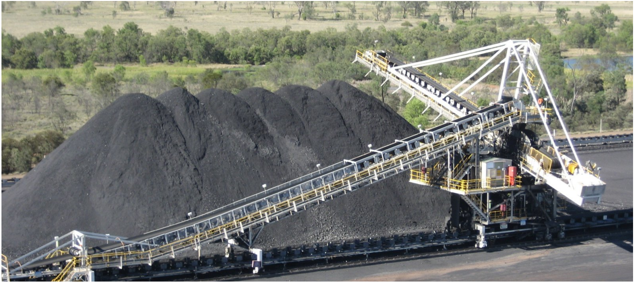
Krupp coal stacker at Kestrel mine. Wikipedia
